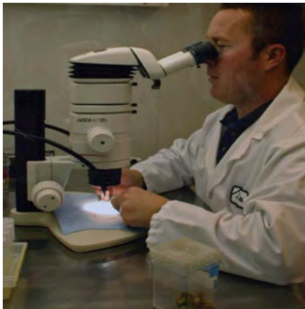
Viewing through a stereoscope, meristem tips are aseptically dissected from daughter plant buds.
