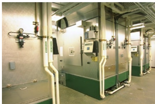
TEMPERATURE, LIGHT AND HUMIDITY are controlled in eight plant growth chambers.
